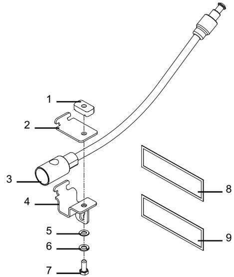
Unlock the cable lock, align the flats on the cable lock with the flats on the lower bracket and insert the cable lock into the lower bracket. Ensure the cable lock housing is fully located into the bracket.
