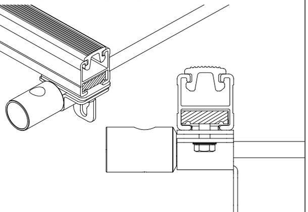
Position the cable lock and bracket assembly, tighten the screw to 5-6Nm to secure the bracket. Peel and stick the yellow warning labels onto the crossbar adjacent to the cable lock.
